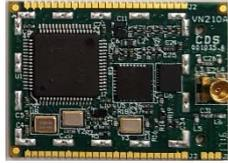
The performed tests validate the design and highlight the advantages of implementing sub 1 GHz ISA100: longer range, lower power consumption, lower design complexity and lower manufacturing costs. Tests for verifying the compliance of the developed system were also performed and the results indicate that the module is compliant with existing standards.
