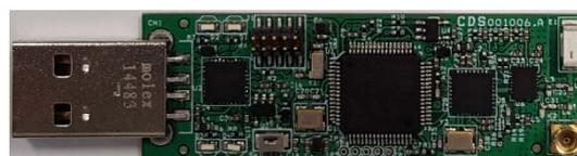
As a secondary result, a VN210A board (replacement for VN210) was obtained. The existing VN210 module produced by the company had to be replaced, because the central IC (microcontroller and transceiver) are no longer manufactured and they disappeared from the market. The new module operating at 2.4 GHz, with the mounted components is shown in the figure below. As soon as ISA100 wireless operating at sub 1 GHz is
