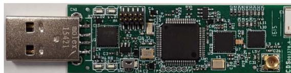
The 2.4 GHz board with the mounted components, developed as an intermediary step, is shown below. It uses the same microcontroller (STM32), and a similar transceiver (Atmel) as the previous one. This platform was used for porting the software implementation, and for simplifying the testing activities, eliminating the uncertainties related to new hardware.
